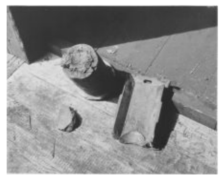
ANOTHER VIEW OF THE SHEARED OFF AXLE END
