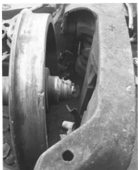
AXLE WITH END SHEARED OFF - CAUSE OF THE WRECK
