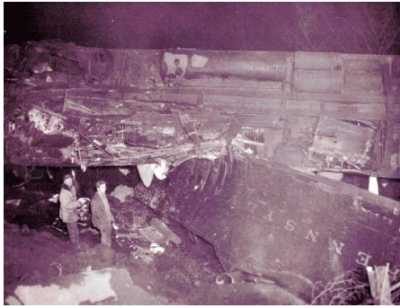
Overturned tender from one of the K4s locomotives at the bottom of the ravine. Greg Sheets - Altoona Archive
