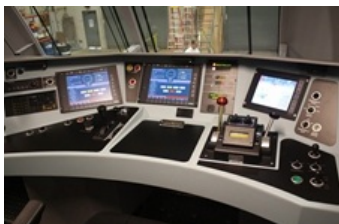
AMTRAK'S MOCK-UP OF THE CONTROL STAND FOR THE AMTRAK CITIES SPRINTER ELECTRIC LOCOMOTIVE. PHOTO BY AMTRAK.
