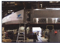
A mechanical lift at the Wilmington mechanical shop holds the first power car to be overhauled.
