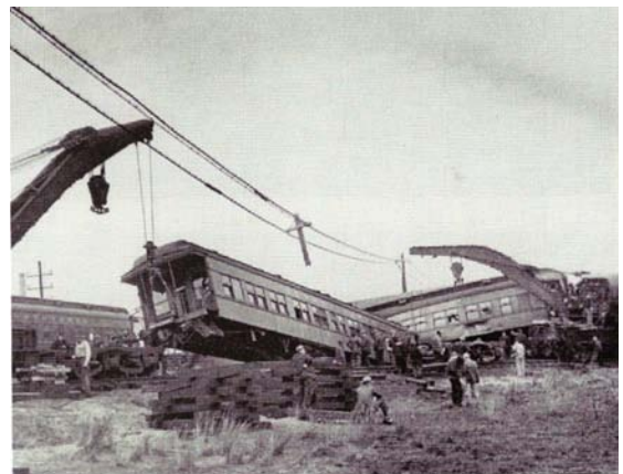
Two steam-powered wrecking cranes lift a slightly damaged type PUW coach. The car's six-wheel trucks have already been placed back on the track.
