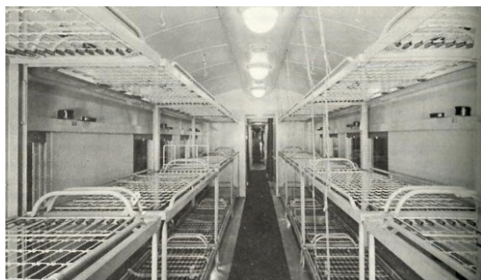
INSIDE VIEW OF NEW SELF-CONTAINED ARMY HOSPITAL CAR WITH THREE-TIER BERTHS ACCOMMODATING 36 PATIENTS
