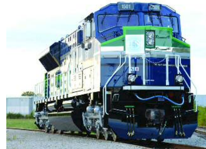
ELECTRO-MOTIVE DIESEL PRE-PRODUCTION SD70ACe-T4 TIER 4 COMPLIANT DIESEL LOCOMOTIVE.
