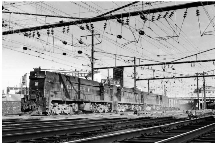
PRR 4439 PASSES THE PRR STATION IN BALTIMORE WITH A SOUTHBOUND FREIGHT IN MARCH 1966. GE BUILT 66 E44 C-C ROAD-SWITCHERS DURING 1960-63 USING THE RECTIFIER TECHNOLOGY PROVEN BY THE BALDWIN-WESTINGHOUSE CAB UNITS. HERBERT H. HARWOOD, JR. PHOTO
