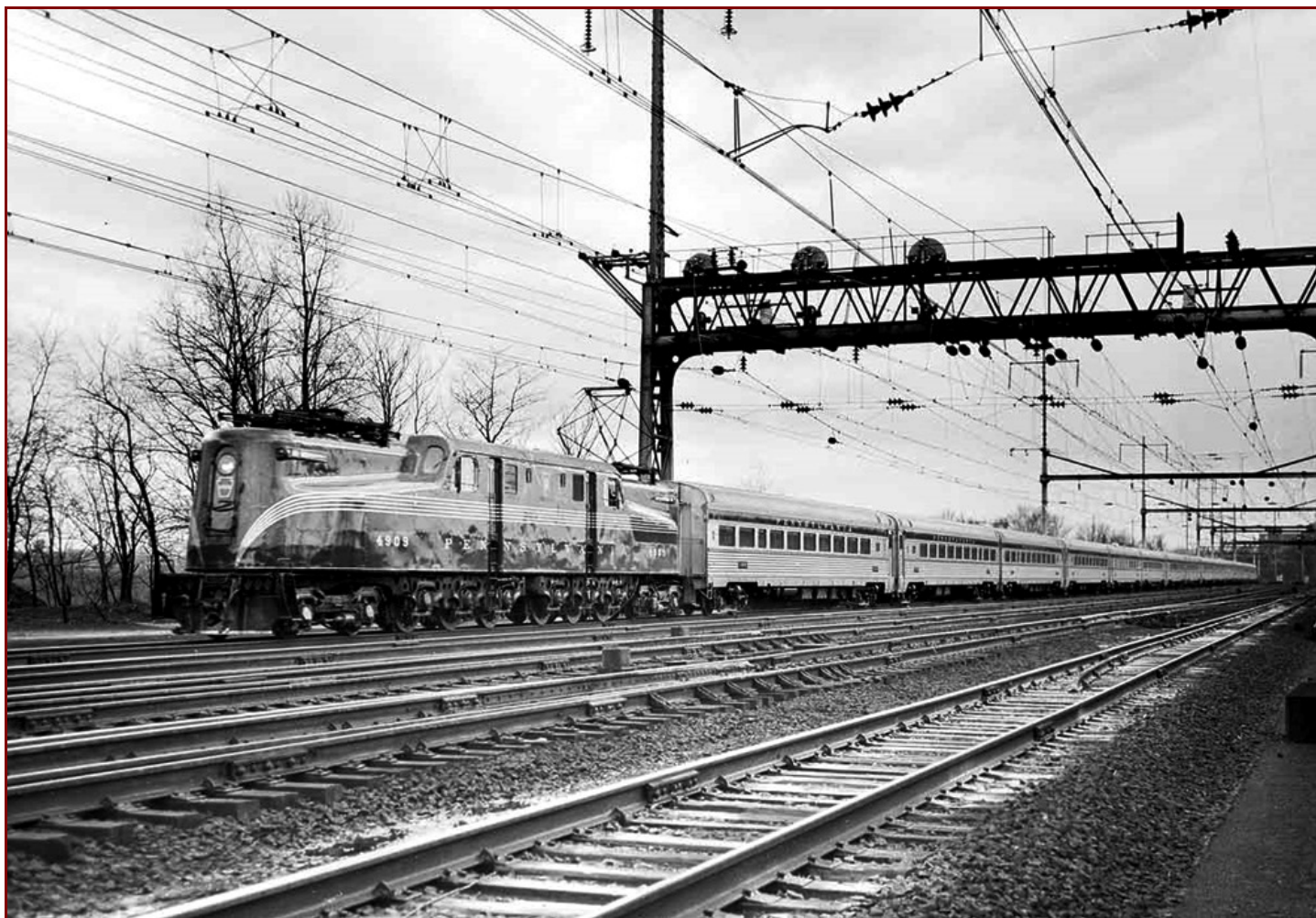
PENNSYLVANIA RAILROAD GG1 No. 4909, ONE OF SEVERAL G'S PAINTED TUSCAN RED FOR SERVICE ON THE NEW CONGRESSIONAL AND SENATOR TRAINS, IS A FEW MINUTES OUT OF 30TH STREET STATION IN PHILADELPHIA WITH THE FIRST RUN OF THE NEWLY RE-EQUIPPED EASTBOUND CONGRESSIONAL ON MARCH 17, 1952 - WAYNE P. ELLIS PHOTO
