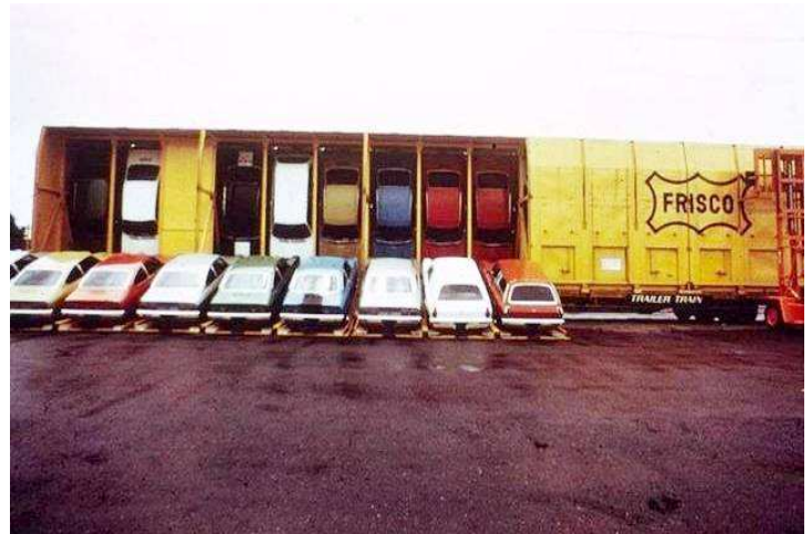
A COMBINATION OF SEDANS AND STATION WAGONS LOADED INTO A ST. LOUIS - SAN FRANCISCO RAILWAY VERT-A-PAC
