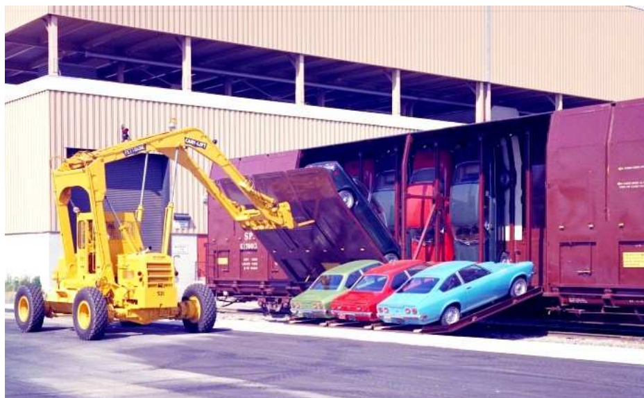
LOADING A SOUTHERN PACIFIC VERT-A-PAC - PHOTO FROM HEMMINGS
