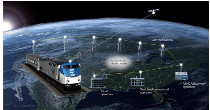
THIS AMTRAK ILLUSTRATION SHOWS HOW PTC TECHNOLOGY WORKS USING LOCOMOTIVES, WAYSIDE EQUIPMENT, AND SATELLITE TECHNOLOGY - AMTRAK
