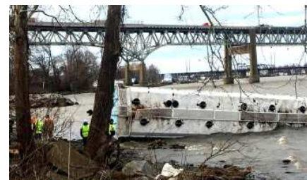
CREWS WORK TO SECURE A COVERED HOPPER CAR THAT FELL FROM THE CSX RAILROAD'S SUSQUEHANNA RIVER BRIDGE DURING FRIDAY NIGHT'S HIGH WINDS AND FLOATED DOWNSTREAM NEAR THE ROUTE 40 HATEM BRIDGE SATURDAY MORNING. ORIGINAL CREDIT: BSMG, TOM SALVATORE - THE ROUTE 40 HATEM BRIDGE IS IN THE FOREGROUND WHILE THE AMTRAK BRIDGE IS IN THE BACKGROUND.
