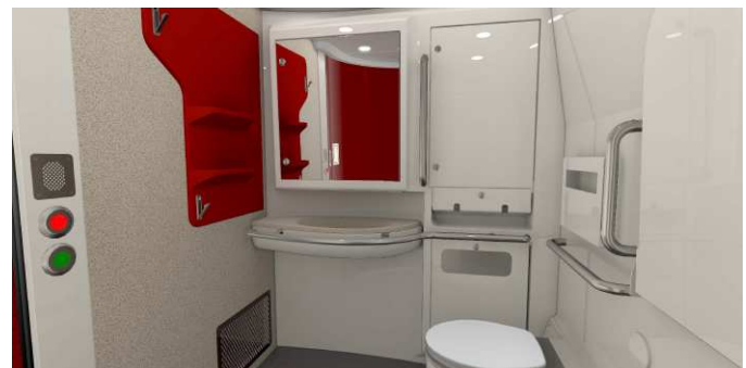
RESTROOM-THE NEW ACELA TRAINSETS FEATURES SPACIOUS ADA-COMPLIANT RESTROOMS WITH A 60-INCH DIAMETER TURNING RADIUS.
