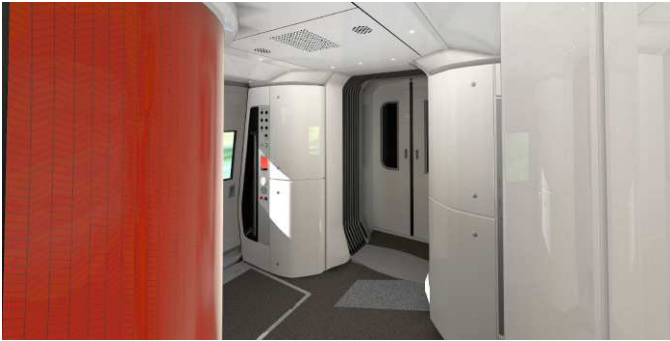
VESTIBULE - THE ARTICULATED DESIGN ALLOWS CUSTOMERS TO EASILY AND SMOOTHLY MOVE BETWEEN TRAIN CARS, WITH LARGE VESTIBULE AREAS.
