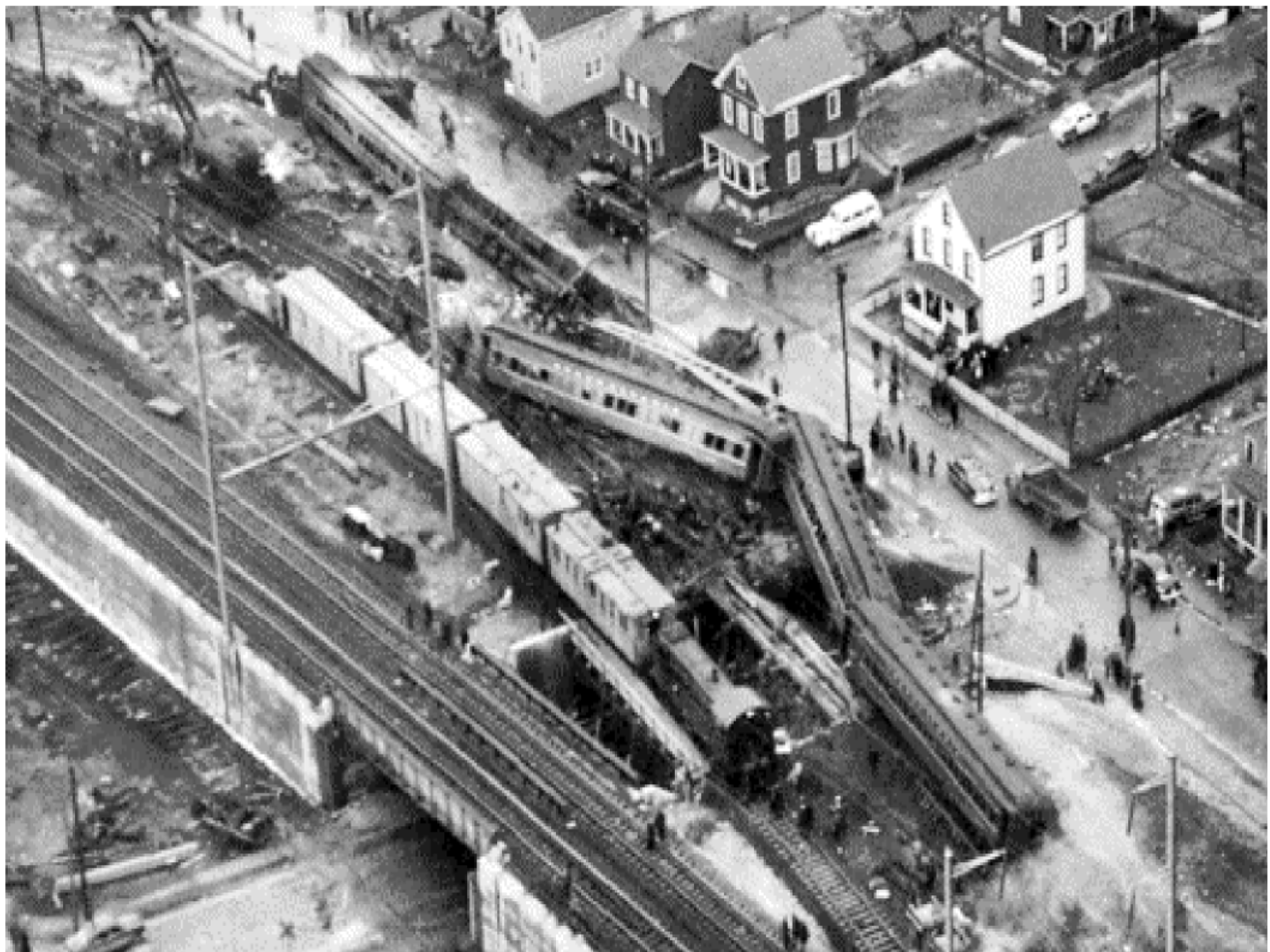
AT 6:06 PM ON SEP. 6, 1943, THE EASTBOUND ADVANCE SECTION OF THE CONGRESSIONAL LIMITED DERAILED AT 56 MPH AT FRANKFORD JCT. IN PHILADELPHIA. THE JOURNAL OF THE 7TH OF 16 CARS BURNED OFF; 6TH-15TH CARS DERAILED; 7TH AND 8TH CAR WERE SLICED OPEN IN A COLLISION WITH A SIGNAL BRIDGE. 79 WERE KILLED. EAST-WEST TRAINS WERE DETOURED VIA THE TRENTON CUTOFF WITH MU SHUTTLES BETWEEN PHILADELPHIA AND HARRISBURG; WASHINGTON TRAINS WERE DETOURED VIA LEHIGH VALLEY-READING AND CRESHEIM BRANCH-TRENTON CUTOFF. DELAIR BRIDGE TRAINS AND SOME CLOCKERS WERE REROUTED TO CAMDEN .(PRR CHRONOLOGY; INTERNET PHOTO)
