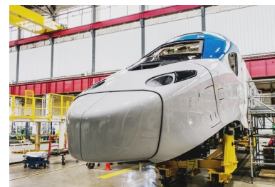
A SIDE-ON VIEW OF AN ALSTOM-BUILT ACELA POWER CAR UNDER CONSTRUCTION AT ALSTOM'S SHOPS IN HORNELL, N.Y. - AMTRAK
