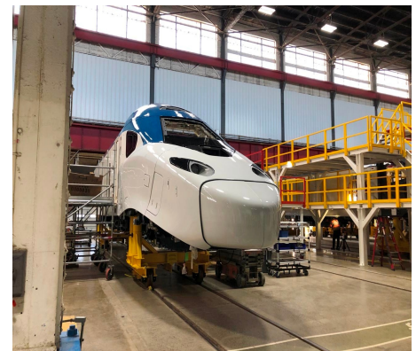
POWER CAR UNDER CONSTRUCTION. EACH TRAINSET WILL CONSIST OF TWO POWER CARS (ONE AT EACH END), SEVEN BUSINESS CLASS COACHES, ONE FIRST CLASS COACH AND A CAFÉ CAR. AMTRAK HAS ORDERED 28 TRAINSETS. THEY ARE EXPECTED TO ENTER REVENUE SERVICE ON THE NORTHEAST CORRIDOR BEGINNING IN 2021.
