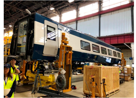
THE TRAINSET IS ARTICULATED, WITH COACHES SHARING A COMMON TRUCK (LIKE THE FRENCH TGV), THEREBY IMPROVING RIDE QUALITY, STABILITY AND SAFETY. BUSINESS CLASS COACHES WILL HAVE GRAY DOORS; FIRST CLASS COACHES WILL HAVE RED DOORS. THE WINDOWS ARE SOMEWHAT TALLER THAN THOSE IN THE EXISTING ACELA EXPRESS EQUIPMENT. THE BLUE AND WHITE LIVERY IS A BIT ON THE RETRO SIDE; IT LOOKS CLOSE TO THE BLUE AND CREAM OF THE FAMOUS CENTRAL RAILROAD OF NEW JERSEY BLUE COMET THAT OPERATED BETWEEN JERSEY CITY AND ATLANTIC CITY IN THE 1930s.
