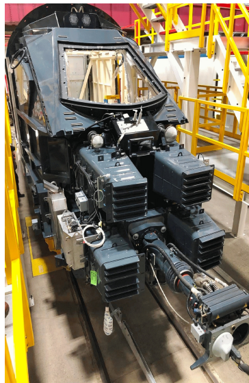
THE TRAINSETS ARE BEING BUILT TO FEDERAL RAILROAD ADMINISTRATION TIER III CRASHWORTHINESS STANDARDS, WITH CEM (CRASH ENERGY MANAGEMENT) TECHNOLOGY. THE PASSENGER COACHES FEATURE OVI (OCCUPIED VOLUME INTEGRITY) CONSTRUCTION, WHEREBY ENERGY TRAVELS THROUGH THE CARBODY STRUCTURE.
