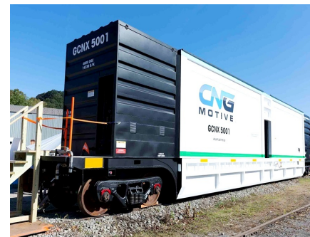
CNGMOTIVE'S NEW, PURPOSE-BUILT COMPRESSED NATURAL GAS TENDER RESEMBLES AN INTERMODAL WELL CAR - CHRIS GUSS
