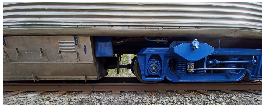
(Left) The direct-drive mechanism of the RDC, who's motors drive one axle at each end of the car. It is a credit to the R&BM shop forces that these early 1950 cars operate so well.
