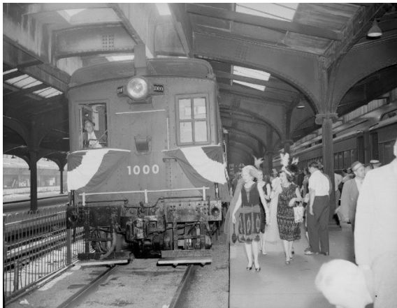
Demonstration run of the Alco M1000 initial diesel Locomotive at Communipaw Terminal – Photo courtesy of the Railroad Museum of Pennsylvania Archives
