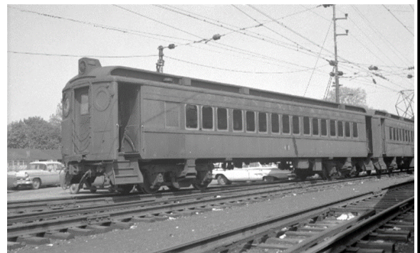
MP 54 Electric Multiple-Unit train near Paoli – Courtesy of the RRMPA
