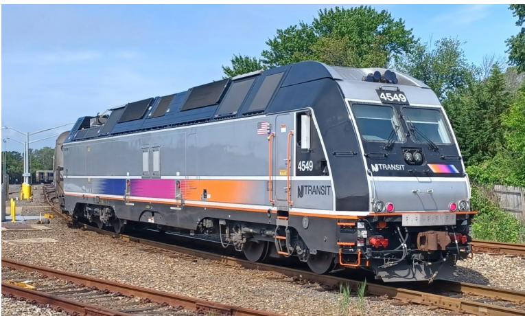
Left: “our” NJY ALP-45DP, # 4549. The “DP” designation refers to dual-power. From Bay Head to Long Branch, the ALP was in diesel-electric mode. Thru trains to northern New Jersey and Manhattan then change to electric pantograph mode as catenary wires originate in Long Branch.
