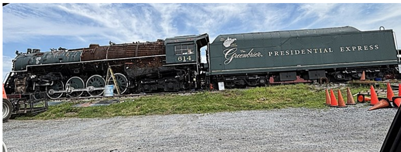
Above: The 614 after inspection work began and its jacket was removed.
