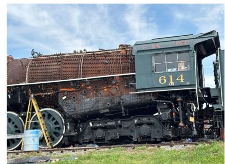
Above: The 614 boiler, firebox, and cab view after inspection work began and its jacket was removed.
